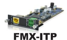
The FMX-ITP is a HDBaseT 1080P seamless input card with audio deembedded signal forFMX system. Paired with a transmitter for transmission of HDMI, IR, RS232, PoH up to 70m.
